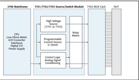
Three source/switch plug-in modules provide
